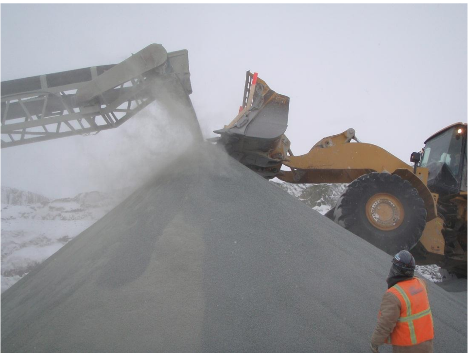
Photo 14: Sampling at the crusher using a plywood box in the loader bucket.
